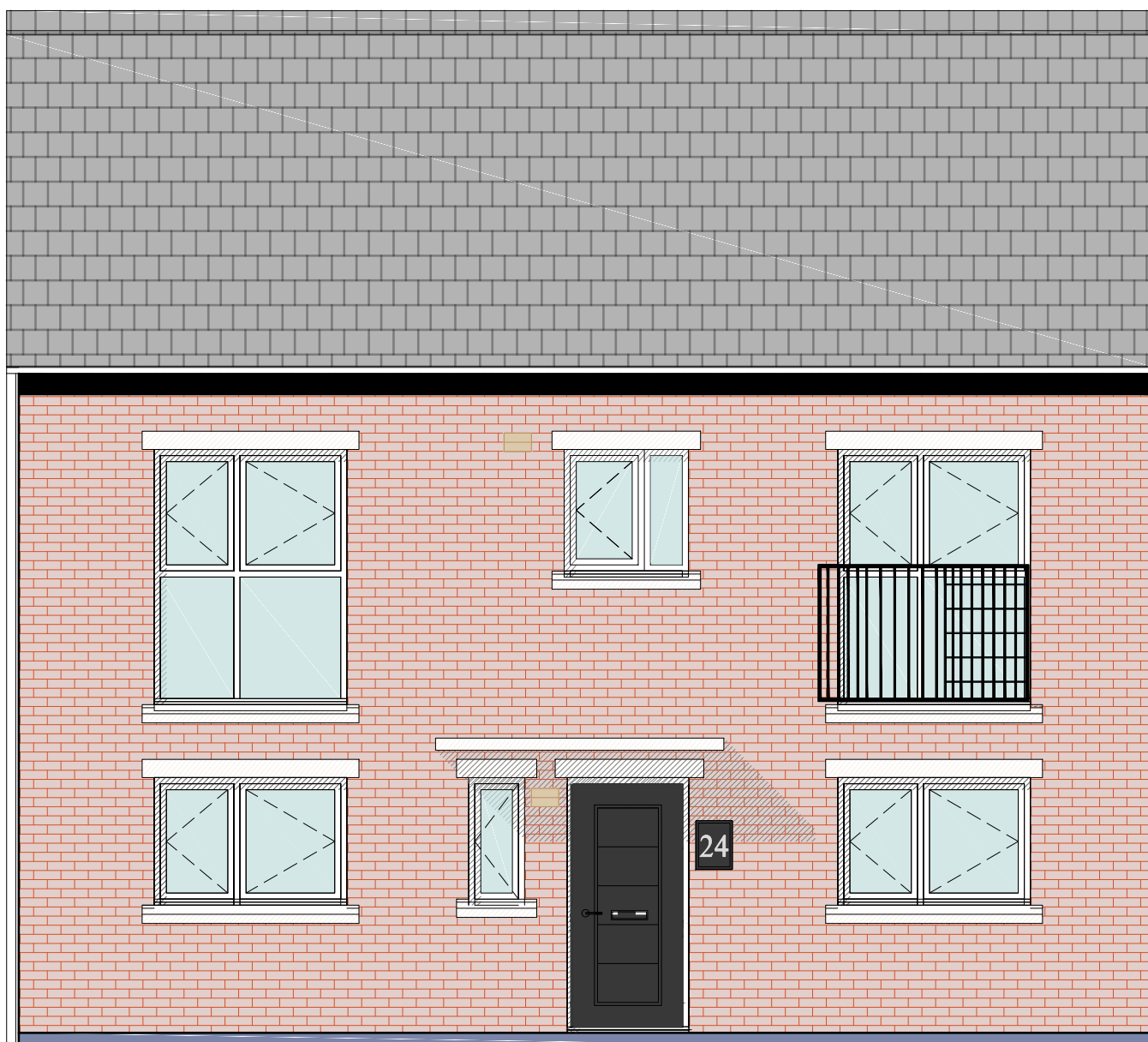
2 BED HOUSE TYPICAL FRONT ELEVATION
